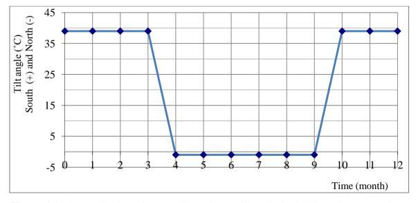
Figure 1.11 Determination of seasonally optimum tilt angle for Minbu solar power plant.
