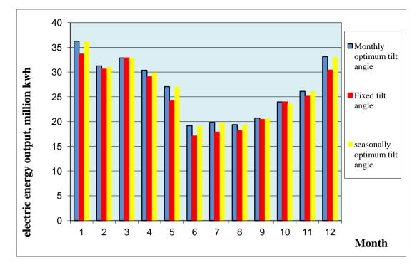
Figure 1.14. Output energy for Minbu solar power plant (fixed, seasonally and monthly optimum tilt angle)
