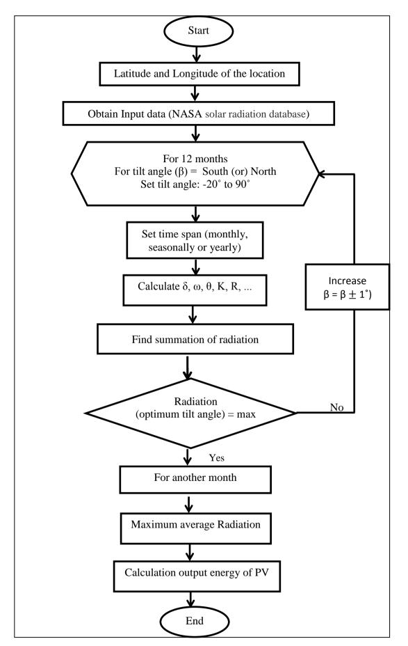
Figure 1.7 Optimization algorithm for PV panels tilt angle.
