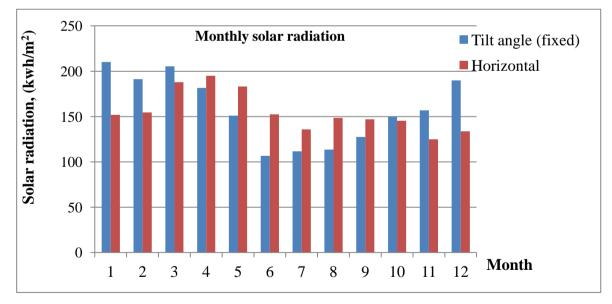
Figure 1.10 (a) Solar radiation for optimum tilt angle for Minbu solar power plant.
