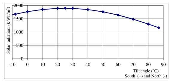
Figure 1.10 (b). Determination of the optimum fixed tilt angle for Minbu solar power plant.
