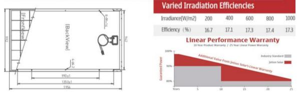
Figure 1.6 Specification of solar panel (JT310) of Minbu solar power plant.
