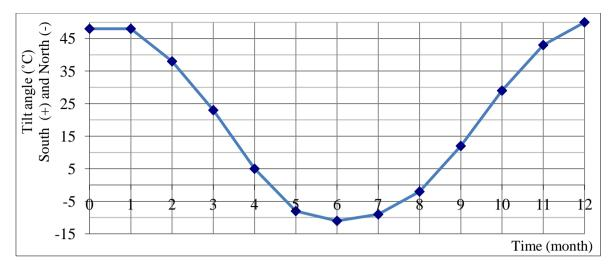
Figure 1.12 Determination of monthly optimum tilt angle for Minbu solar power plant
